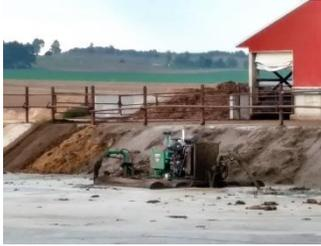
A John Deere “manure boat” is essentially a large air compressor outfitted with nozzles. It homogenizes the solids and the liquids so that they can be hauled and spread on crop fields where it can provide both nutrients and organic matter to the soil.
