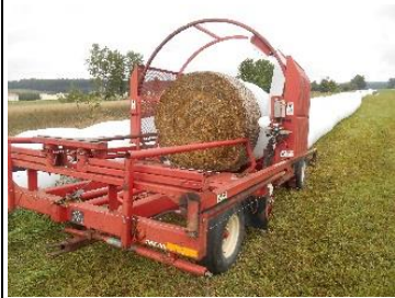
Individual bales of hay are first wrapped in netting to hold them together, and then in plastic film to enable them to ferment.
